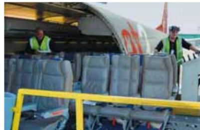
During the year to 31 March 2006, the Group increased its owned aircraft fleet to 21 Boeing 737-300 aircraft, which carry 148 passengers, and three Boeing 757-200s, which carry 235 passengers. Since the year end two further Boeing 757-200s have been purchased. Of the Boeing 737-300s, six are “Quick Change” versions, allowing the seats to be removed and containers of mail to be loaded within 40 minutes, for Royal Mail’s “Postal Air Network”.
